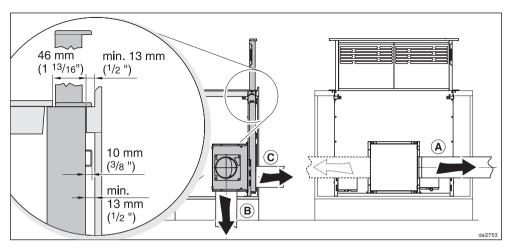
Exhaust air ducting using the DAG 500 internal blower, installed on the front of the appliance [vent duct 6" Ø (150 mm)]: (a) to the left or right, (b) downwards, (c) to the rear.
